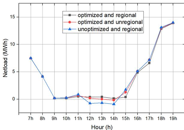
Fig. 11. Aggregated netload profile of all the prosumers.
