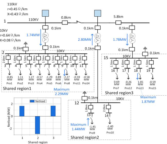
Fig. 8. Load distribution and main power flow in time slot 13.
