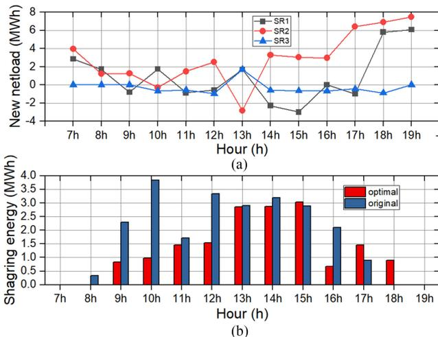
Fig. 6. Optimized netload and its standard deviation compared with the original. (a) New netload. (b) Sharing energy.
