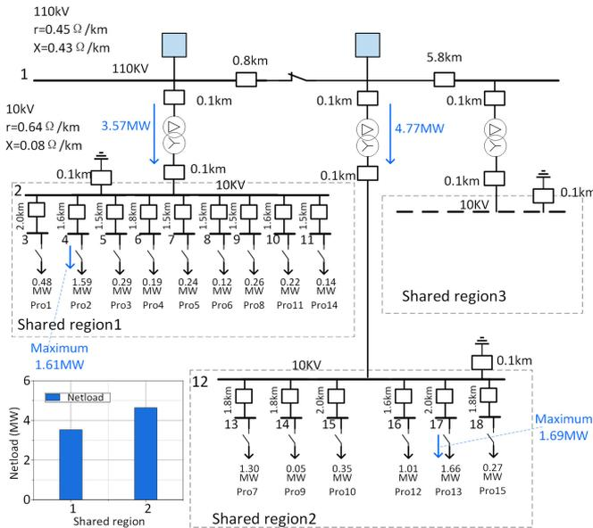
Fig. 7. Load distribution and main power flow in time slot 7.
